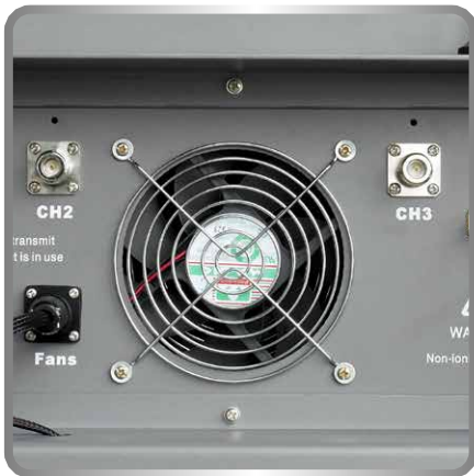
Active Cooling System
